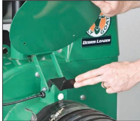
**Safety kill switch** Quick connect / release hose clamp with safety interlock.
