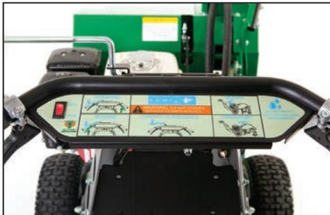
**Self-propelled, variable speed**, intuitive hydro-drive controls allow you to feather the speed and aerate in both forward and reverse with finger tip control. Reduces fatigue and vibration. Takes the chore out of the chore!
