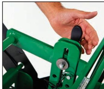
**Set and Forget™ blade depth adjustment to 2.5"** Single lever and clamp at user's operating position adjusts simply, saving time and providing precise cutting depths.
