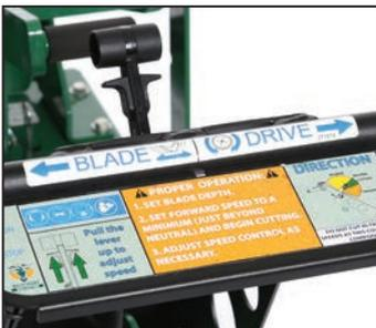
**Hydro drive transmission** Variable speed hydrostatic drive allows user to tailor cutting speed to ground condition, maintaining sod quality and maximising productivity. Adjustable reverse speed allows seamless manoeuvring out of tight areas quickly, without damaging turf.
