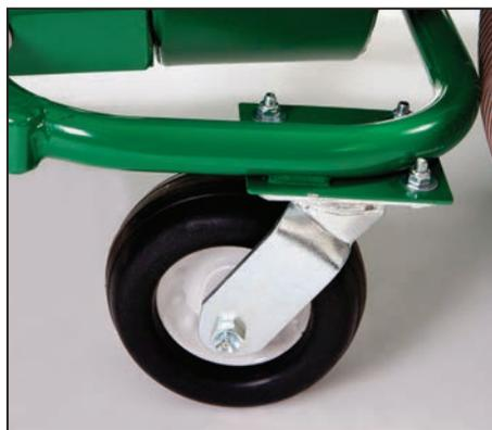
**Durable front casters** roll smoothly through turns and over uneven surfaces offering quick task completion.
