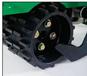
**Unique drive wheels** Tough cutting conditions are easily executed as paddle style wheels clear mud and improve grip for added control.
