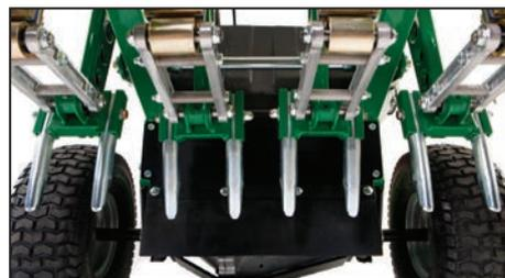
**Fast tine service** Only 8 tines and 4 bolts which are easily accessed and takes 10% of the time needed to service 40+ tine, 2-bolt drum units.
