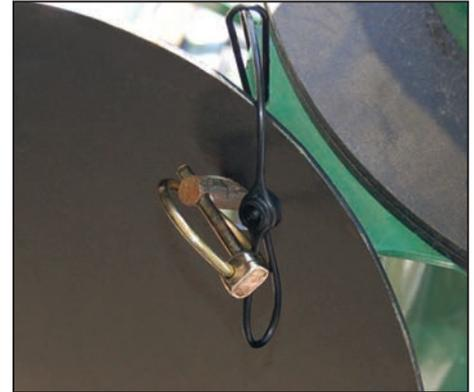
**Intake hose storage** Simple secure nozzle hook for convenient and efficient storage.
