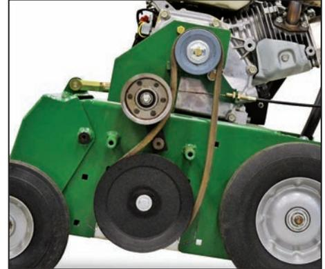
**Premium pulleys**, easy to adjust idler, and easy to change belt contribute to simple service and long life. Protected by a steel guard.
