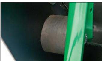
**Multiple oversized isolation mounts** are designed to absorb vibration so operator completes tasks quickly, comfortably and without fatigue.
