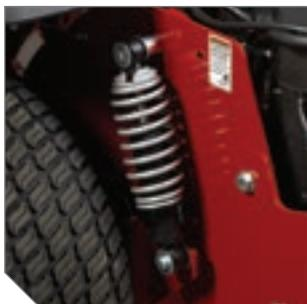
**Exclusive suspension system** consists of rear coil-over-shocks (shown) and pivoting front axle with shocks.
