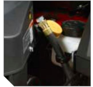
Convenient oil dump hose will make oil changes fast with less mess.
