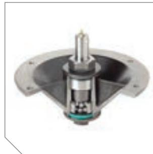
**Hercules II Spindles** industrial 10" dia. cast-iron spindle assembly with 1 3/16" dia. shaft and greasable double row angular contact ball bearings, which can be greased through the convenient top access grease fitting.
