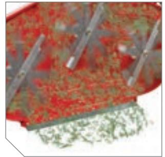
**Rear-discharge decks**, used for special applications, disperse grass clippings directly behind the mower.
