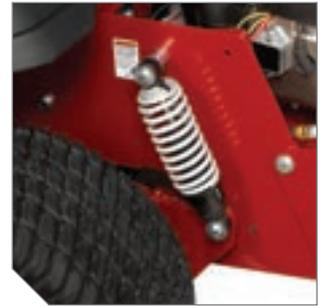
**Exclusive suspension system** consists of rear coil-over-shocks (shown) and pivoting front axle with coil-over-shocks.
