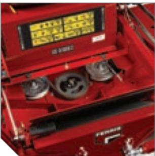
**Removable floor pan** provides access to the top of the deck for easy cleaning and service.
