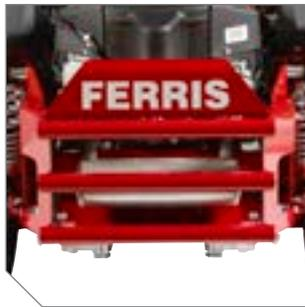
Rugged rear bumper protects the engine compartment
