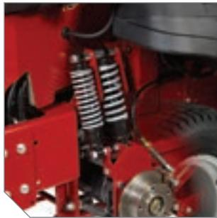
**Exclusive suspension system** consists of dual rear coil-over-shocks with dual suspension arms (shown) and front independent adjustable coil-over-shocks.
