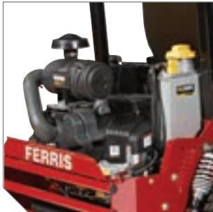
**NEW!** Oil Guard System with extended oil change intervals — 500 hours on Vanguard BIG BLOCK™ engine.
