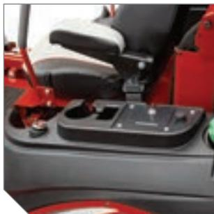
**Operator compartment** includes ergonomic control panels, a cup holder, mobile phone pocket, 12-volt outlet and storage compartment.
