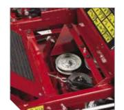
Quick removal of the **floor pan** provides convenient access to the top of the deck for easy cleaning and service.
