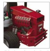
Noise-dampening engine shroud absorbs and reduces noise for improved operator and bystander comfort.
