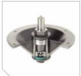
**Hercules**™ **II Spindles** industrial 10" dia. cast-iron spindle assembly with 1 <sup>3</sup>/<sub>16</sub>" dia. shaft and greaseable double row angular contact ball bearings, which can be greased through the convenient top access grease fitting.
