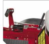
Foot-operated deck lift, with adjustable pedal, can change cut height in 1/4" increments from 1.5"- 5".
