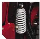
**Exclusive suspension system** consists of adjustable rear coil-over-shocks (shown) and front independent adjustable coil-over-shocks.
