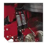
**Exclusive suspension system** consists of dual rear coil-overshocks with dual suspension arms (shown) and front independent adjustable coil-over-shocks.
