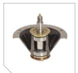
Cast-Iron Spindles longer usable life, 1" shaft with top access grease fitting for greaseable dual ball bearings, six-bolt 8" flange design adds strength and greater dispersal of energy to deck assembly. (61" models)
