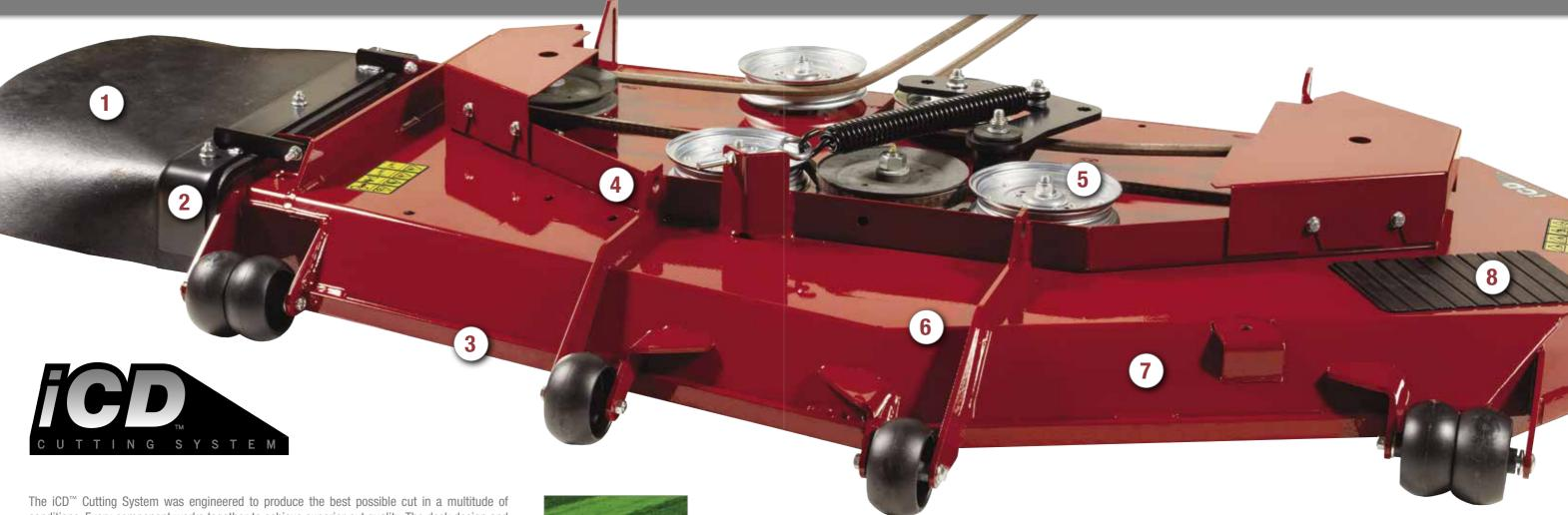
conditions. Every component works together to achieve superior cut quality. The deck design and extra wide discharge opening allow for a more even and greater dispersal of clippings. The shell features a sloped nose design which allows the blades of grass to rise in the chamber before making contact with the blades and also reduces the amount of clippings that are discharged from the front. Slice through thick grass with ease and get the job done sooner than you expected.
