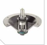
Hercules™ II Spindles industrial 10" dia. cast-iron spindle assembly with 1 3/16" dia. shaft and greaseable double row angular contact ball bearings, which can be greased through the convenient top access grease fitting.
