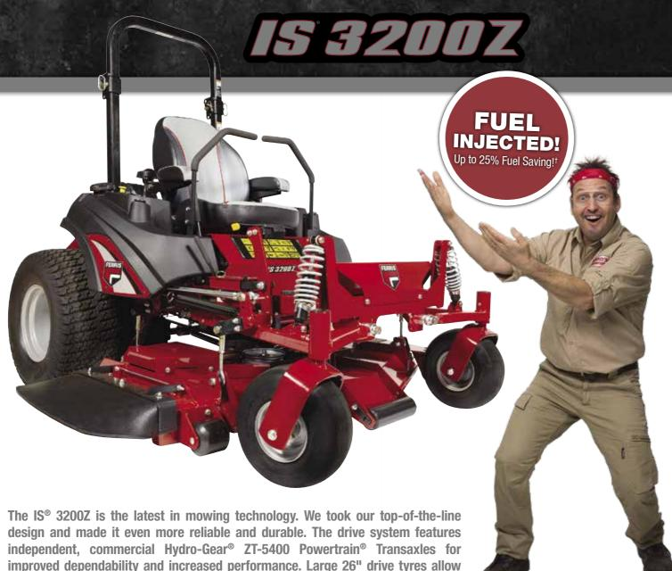
improved dependability and increased performance. Large 26" drive tyres allow for greater traction, smoother ride and improved curb climbing performance. The deck mounting and levelling systems have been updated with solid steel hangers for added reliability and ease of adjustment.
