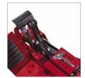
Foot-operated deck lift, with adjustable pedal, can change cut height in 1/4" increments from 1.5"- 4.5".
