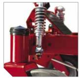
The Suspension Comfort System<sup>™</sup> (SCS<sup>™</sup>) complete with front and rear springs allows the operator to feel 25% less impact° while operating resulting in enhanced comfort versus nonsuspension zero-turn mowers.‡
