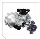
The **ZT-2800**® is Hydro-Gear®'s premium transaxle with charge **pumps** providing tough and smooth operation for larger properties.
