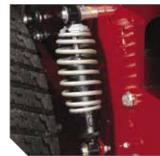
**Exclusive suspension system** consists of adjustable rear coil-over-shocks (shown) and front independent adjustable coil-over-shocks.
