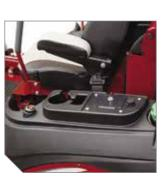
**Operator compartment** includes ergonomic control panels, a cup holder, mobile phone pocket, 12-volt outlet and storage compartment.
