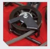
A. Belt Guide Steel arms help prevent belt from dislodging from serviceable cast-iron backside idler with dust shield.
