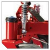
The Suspension Comfort System (SCS<sup>™</sup>) complete with front and rear springs allows the operator to feel 25% less impact<sup>o</sup> while operating resulting in enhanced comfort versus nonsuspension zero-turn mowers.<sup>‡</sup>
