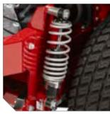
Patented suspension system consists of adjustable rear progressive coil-over-shocks (shown) and front adjustable coil-over-shocks.
