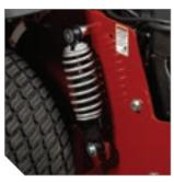
Exclusive suspension system consists of rear coil-over-shocks (shown) and pivoting front axle with shocks.
