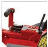
**Foot-operated deck lift**, with adjustable pedal, can change cut height in 1/4" increments from 1.5"- 5".
