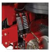
**Exclusive suspension system** consists of dual rear coil-overshocks with dual suspension arms (shown) and front independent adjustable coil-over-shocks.
