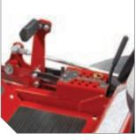
Foot-operated deck lift, with adjustable pedal, can change cut height in 1/4" increments from 1.5"- 5".
