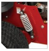
Exclusive suspension system consists of rear coil-over-shocks (shown) and pivoting front axle with coil-over-shocks.
