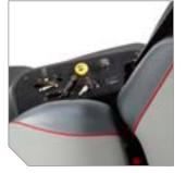
Ergonomic control panel with dual channel hour meter and parking brake.
