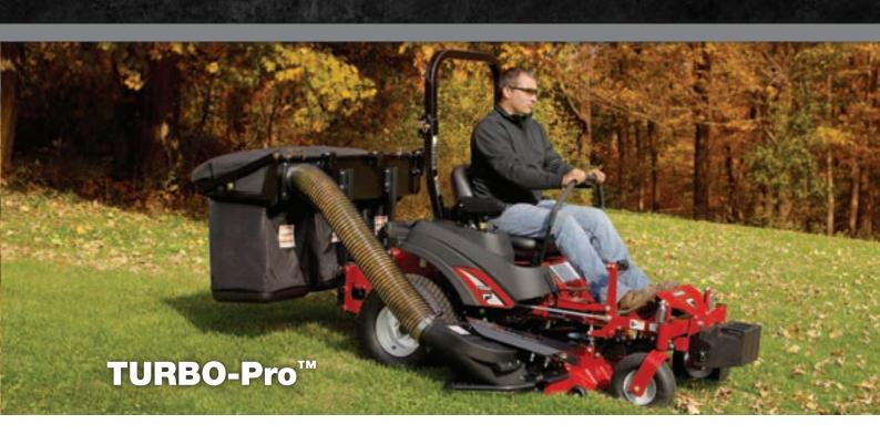
The TURBO-Pro<sup>™</sup> System makes collecting leaves and debris a breeze. This lightweight blower assembly is ideal for use with compact models.
