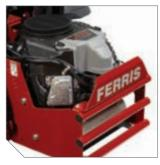
Heavy-duty bumper protects the engine while also allowing for easy service access.
