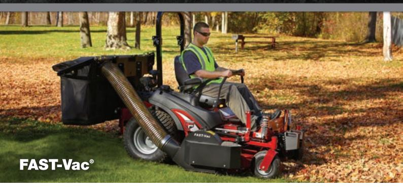
The FAST-Vac<sup>®</sup> System is built around a tough, high-volume side panel air induction system that reduces clogging and produces significantly more air volume than conventional systems. The rugged impeller utilizes industrial-grade bearings, generates phenomenal airflow. Its spindle-driven vertical turbo is narrower, allowing you to get in and out of tight places.
