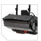
**Electric DFS** Simply flip the switch on the control panel to release the hopper right from your seat. Capacity: 13 cubic feet
