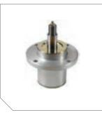
Aluminium Spindles feature 1" shaft with greaseable 2.5" x 1" dual ball bearings with top access grease fittings and pressure relief valve.
